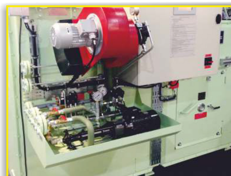
Roto Pump feeding dirty oil for incineration
