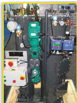
Roto Pump feeding oily water on OWS
